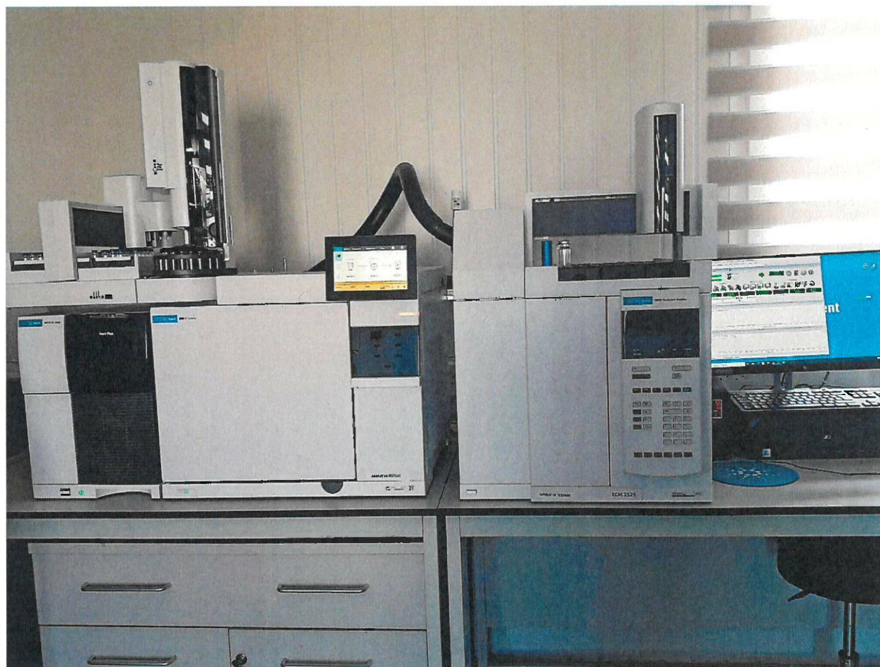
GC-MS (aparat determinari pesticide, PAH, BTEX, COV)
