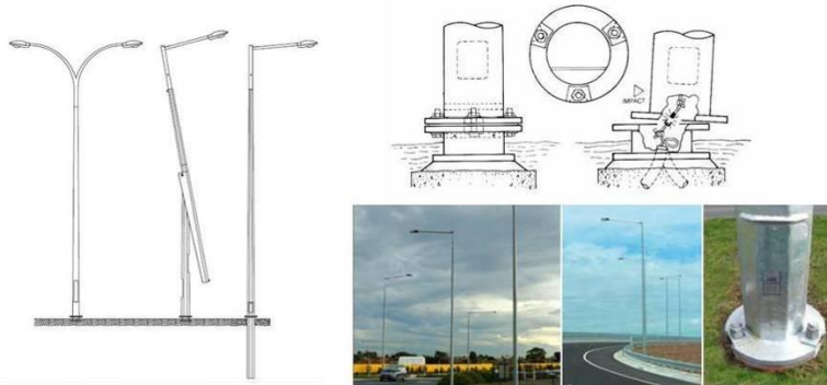
Figura 24: Stâlpi de tip “rupere de la bază” (Source: Department of infrastructure, Energy and Resources: Road Hazard Management Guide, Tasmania, 2014)
